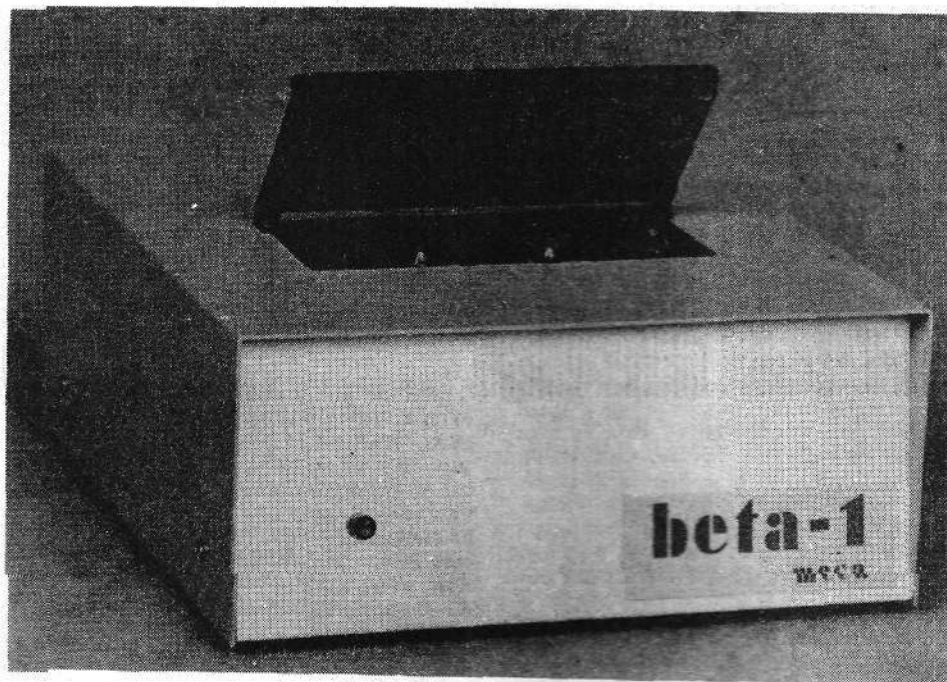
Beta-1—High-speed tape for TRS-80 stores one megabyte, with 10 second average access time.
