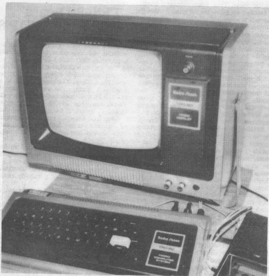
LOOK MA: LESS CORDS —Power supply in this setup has been hidden away in the video monitor, just under the Radio Shack medallion. Monitor also has been raised off table with a "U" bracket, which allows it to swivel.
