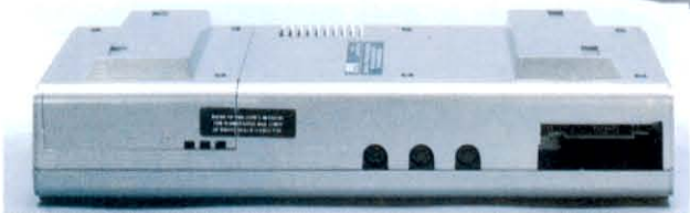
Rear outlets for power supply cords, cassette and disk drive cables.
