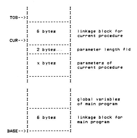
With the three data stack pointers, the parameters passed to the procedure can be accessed. If it is a function the return value can be stored. Also the global variables of the main program can be accessed. For example, if the first global variable declared in the main Pascal program which calls the external procedure is an integer named INT1 then just add 6 to the BASE pointer to get the address of INT1. The BASE pointer is in register pair HL on entry to the procedure.
